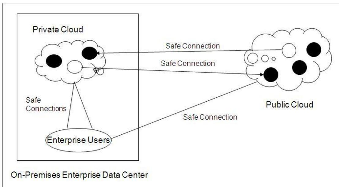
The black circles in the illustration represent active virtual server images and the white circles represent virtual server images that have been migrated (using safe connections). The arrows indicate the direction of migration. Enterprise users are connected to the clouds using safe connections, which can be virtual private networks (VPNs) or secure HTTP browsers.
